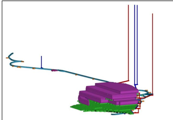
SLC production crosscuts have primarily been designed so that each level is horizontally offset from the level above and below. The design parameters for the SLC production drives at Cactus East and Parks/Salyer are in line with other SLC operations.
